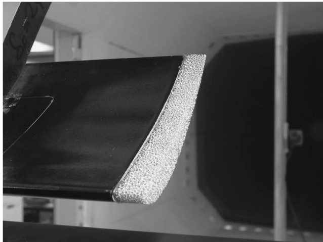
Fig. 3 A downstream view of the porous flap side edge. The PIV camera can be seen mounted on the strut in the background. The laser sheet shines from right to left in a vertical plane.
